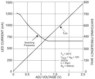
Figure 5 Buck LED Current, Switching Frequency vs.  $V_{ADJ}$
