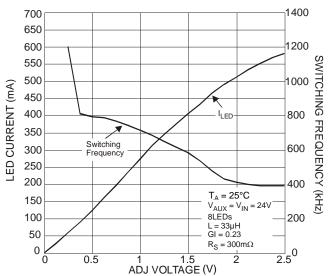
Figure 6 Buck-Boost LED Current, Switching Frequency vs.  $V_{ADJ}$
