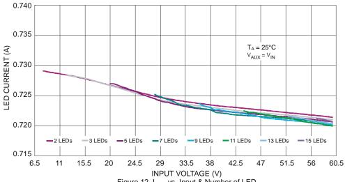
Figure 12 I<sub>LED</sub> vs. Input & Number of LED
