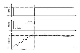
Figure 36 Diagnostic During Start-Up
