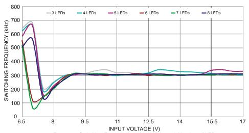
Figure 19 Switching Frequency vs. Input Voltage & Number of LED
