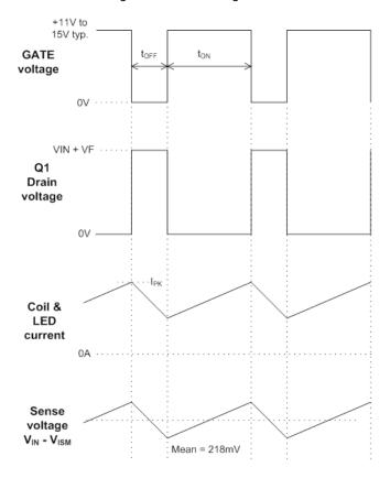
Figure 22 Operating Waveforms (Buck Mode)
