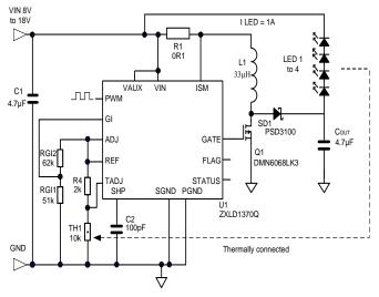
Buck-Boost Diagram Utilizing Thermistor and TADJ
