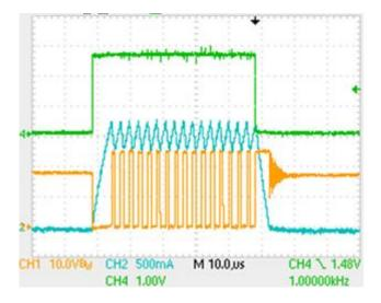
The PWM pin can be used to put the device into standby. Taking the PWM pin low (<0.4V) for more than 25ms (typically 15ms) the device will enter its standby state and most of the internal circuitry is switched off and residual quiescent current will be typically 90 $\mu$ A. In particular, the STATUS pin will go down to GND while the FLAG and REF pins will stay at their nominal values.
