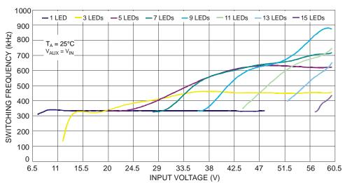
Figure 10 Frequency vs. Input Voltage & Number of LED
