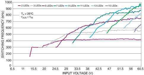
Figure 13 Frequency ZXLD1370Q - Buck Mode - L47µH
