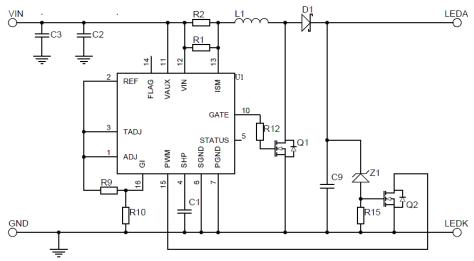
Figure 43 Application Circuit - 400mA Boost LED Driver
