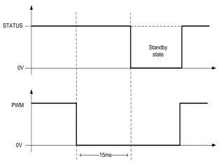
Figure 33 Standby State from PWM Signal
