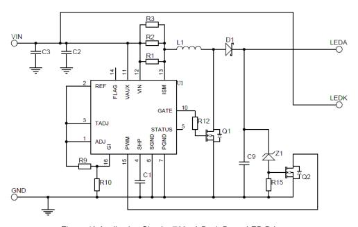
Figure 46 Application Circuit - 700mA Buck-Boost LED Driver
