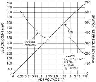
Figure 7 Boost LED Current, Switching Frequency vs.  $V_{\rm ADJ}$
