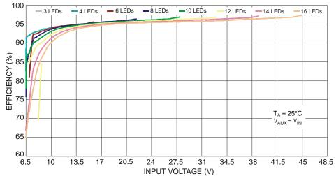
Figure 17 Efficiency vs. Input Voltage & Number of LED
