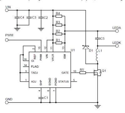
Figure 40 Application Circuit: 2.8A Buck LED Driver
