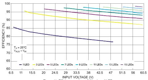
Figure 11 Efficiency vs. Input & Number of LED
