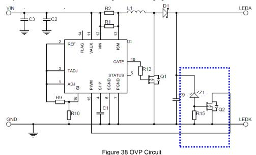
The Zener voltage is determined according to: V<sub>Z</sub> = V<sub>LEDMAX</sub> +10% where V<sub>LEDMAX</sub> is maximum LED chain voltage.
