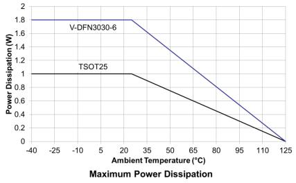
Note that the device power dissipation will most often be at maximum at minimum supply voltage. It will also increase if the efficiency of the circuit is low. This may result from the use of unsuitable coils, or excessive parasitic output capacitance on the switch output.
