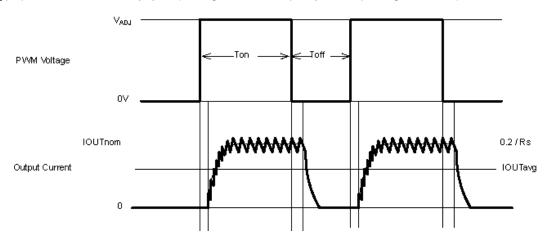
Figure 4 Low Frequency PWM Operating Waveforms
