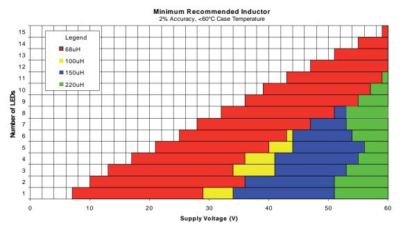
Figure 3. ZXLD1356Q Minimum Recommended Inductor
