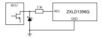
If the NMOS transistor within the microcontroller has high Gate/Drain capacitance, this arrangement can inject a negative spike into ADJ input of the ZXLD1356Q and cause erratic operation. The addition of a Schottky clamp diode (e.g. Diodes Inc. SD103CWS) to ground and inclusion of a series resistor (3.3k) will prevent this. See the section on PWM dimming for more details of the various modes of control using high-frequency and low-frequency PWM signals.
