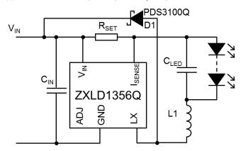
A value of 1µF will reduce the supply ripple current by a factor three (approximately). Proportionally lower ripple can be achieved with higher capacitor values. Note that the capacitor will not affect operating frequency or efficiency, but it will increase start-up delay, by reducing the rate of rise of LED voltage.
