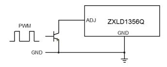
This scheme uses the 50k resistor between the ADJ pin and the internal voltage reference as a pull-up resistor for the external transistor (e.g. Diodes Inc. MMBT3904).
