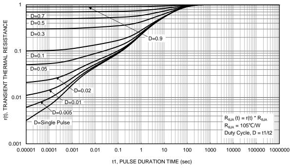
Figure 13. Transient Thermal Resistance
