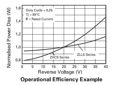
The operational efficiency chart indicates the beneficial use of the ZLLS series diodes in applications requiring higher voltage, higher temperature operation. Circuits requiring low voltage low temperature operation will benefit from using Zetex low  $V_F$  ZHCS series diodes.
