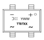
TT8TXX = Product Type Marking Code XX = 06 or 08 )'.'= Manufacturer's Code Marking YWW = Date Code Marking Y = Last Digit of Year (ex: 3 = 2023) WW = Week Code (01 to 53)
