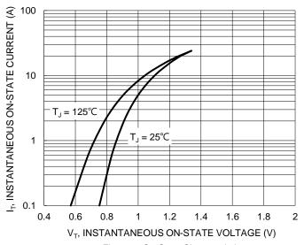
Figure 6. On-State Characteristics
