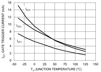
Figure 1. Typical Gate Trigger Current vs. Junction Temperature
