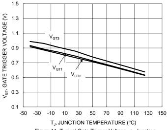
Figure 11. Typical Gate Trigger Voltage vs. Junction Temperature
