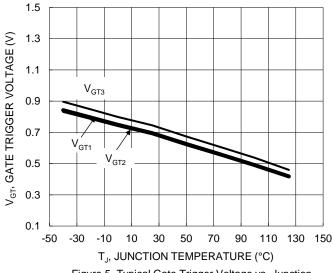
Figure 5. Typical Gate Trigger Voltage vs. Junction Temperature
