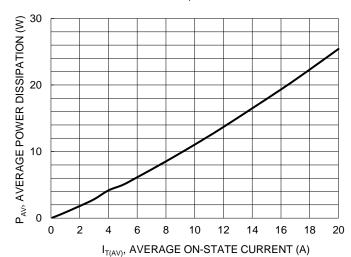
Figure 4. On-State Power Dissipation
