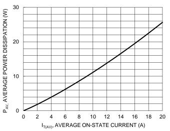
Figure 10. On-State Power Dissipation
