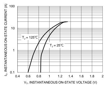
Figure 12. On-State Characteristics
