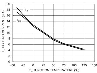
Figure 2. Typical Holding Current vs. Junction Temperature
