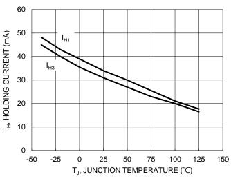
Figure 8. Typical Holding Current vs. Junction Temperature
