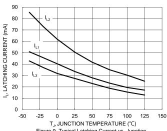
Figure 9. Typical Latching Current vs. Junction Temperature
