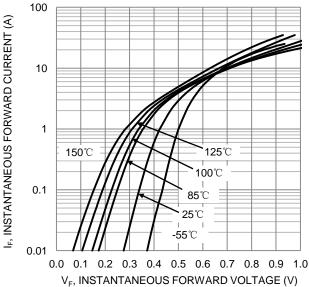
Figure 2. Typical Forward Characteristics
