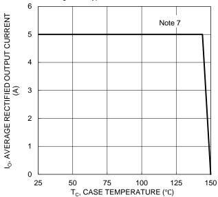
Figure 5. DC Forward Current Derating
