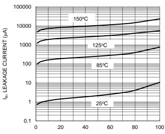
$V_{\rm R}$ , REVERSE VOLTAGE (V) Figure 3. Typical Reverse Characteristics
