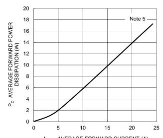
I<sub>F(AV)</sub>, AVERAGE FORWARD CURRENT (A) Figure 1. Forward Power Dissipation
