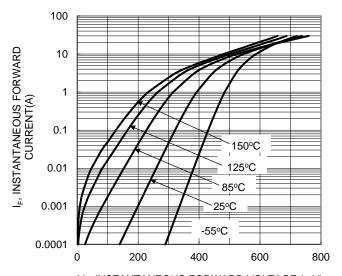
V<sub>F</sub>, INSTANTANEOUS FORWARD VOLTAGE (mV) Figure 2. Typical Forward Characteristics
