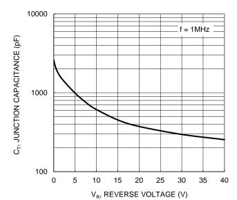
Figure. 5 Typical Junction Capacitance
