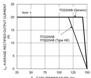
$T_{\rm C}$ , CASE TEMPERATURE (°C) Figure 4 DC Forward Current Derating
