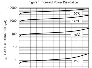
V<sub>R</sub>, REVERSE VOLTAGE (V) Figure 3. Typical Reverse Characteristics
