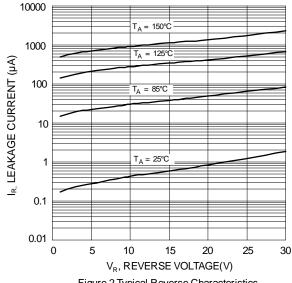
Figure 2 Typical Reverse Characteristics
