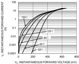
Figure 2. Typical Forward Characteristics
