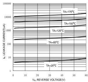
Figure.2 Typical Reverse Characteristics
