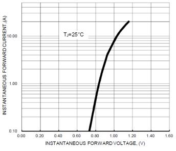
FIG.3- TYPICAL FORWARD CHARACTERISTICS
