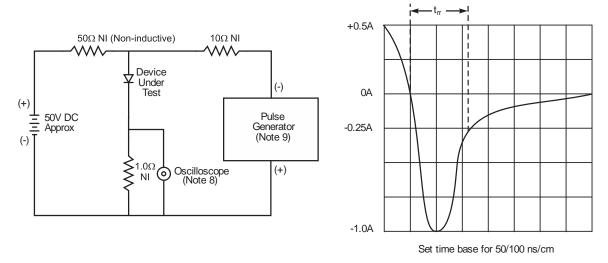
Figure 7 Reverse Recovery Time Characteristic and Test Circuit
