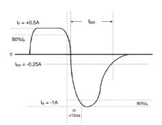
Figure 7 Reverse Recovery Time Characteristics and Test Circuit
