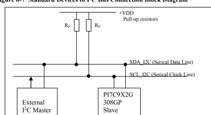
Figure 6-7 Standard Devices to I<sup>2</sup>C Bus Connection Block Diagram
