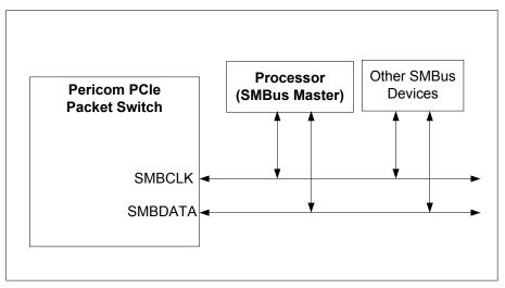
The SMBus interface on the Packet Switch consists of one SMBus clock pin (SCL\_I2C), a SMBus data pin (SDA\_I2C), and 3 SMBus address pins (GPIO[7:5]). The SMBus clock pin provides or receives the clock signal. The SMBus data pin facilitates the data transmission and reception. Both of the clock and data pins are bi-directional. The SMBus address pins determine the address to which the Packet Switch responds to. The SMBus address pins generate addresses according to the following table:
