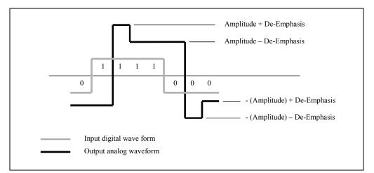
Figure 5-1 Driver Output Waveform
