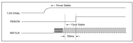
Figure 10-1 Initial Power-Up Sequence
