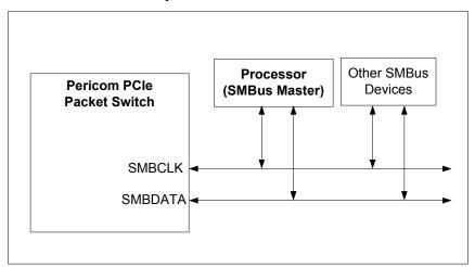
The SMBus interface on the PI7C9X2G304EL consists of one SMBus clock pin (SMBCLK), a SMBus data pin (SMBDATA), and 3 SMBus address pins (GPIO[5:7]). The SMBus clock pin provides or receives the clock signal. The SMBus data pin facilitates the data transmission and reception. Both of the clock and data pins are bi-directional. The SMBus address pins determine the address to which the PI7C9X2G304EL responds to. The SMBus address pins generate addresses according to the following table:
