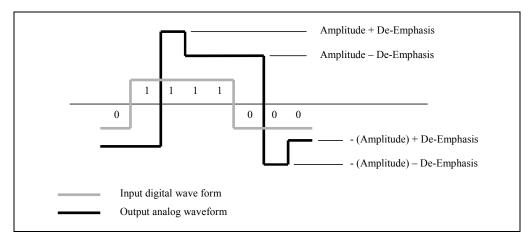
Figure 5-1 Driver Output Waveform
