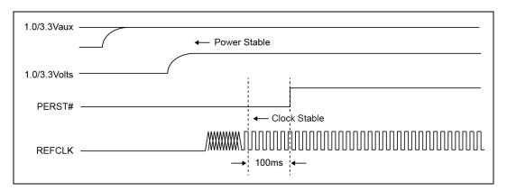
Figure 11-1 Initial Power-Up Sequence
