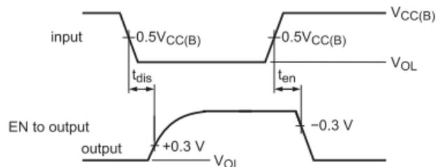
Figure 4: Propagation Delay and Enable and disable time
