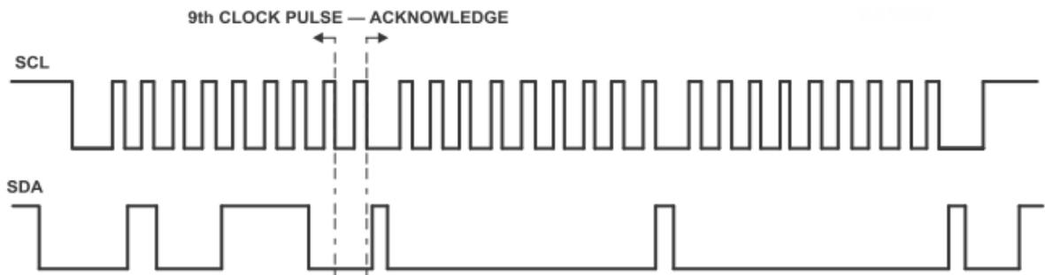
Figure 9: Bus A (0.6V to 5.5V Bus) Waveform
