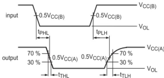
Figure 2: Propagation Delay and Transition Times B → A
