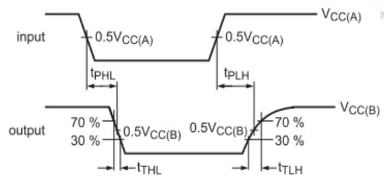
Figure 3: Propagation Delay and Transition Times A → B
