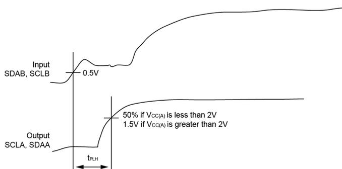
Figure 4: Propagation Delay
