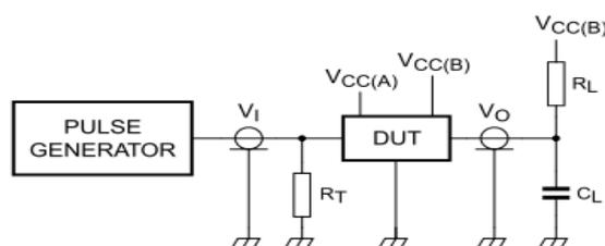
$R_L$  = Load resistor: 1.35kΩ on port B; 167Ω on port A (0.8V to 2.7V) and 450Ω on port A (3.0V to 5.5V)
