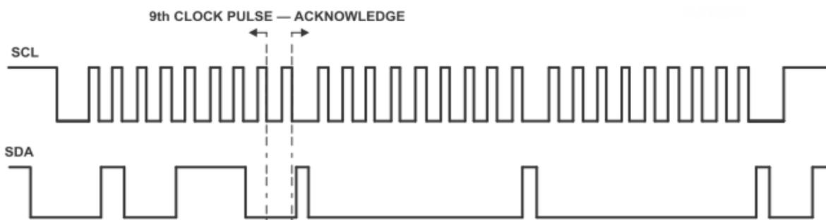
Figure 9: Bus A (0.8V to 5.5V Bus) Waveform
