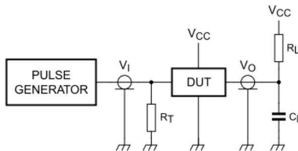
$R_L$  = load resistor; 1.35 k $\Omega$
