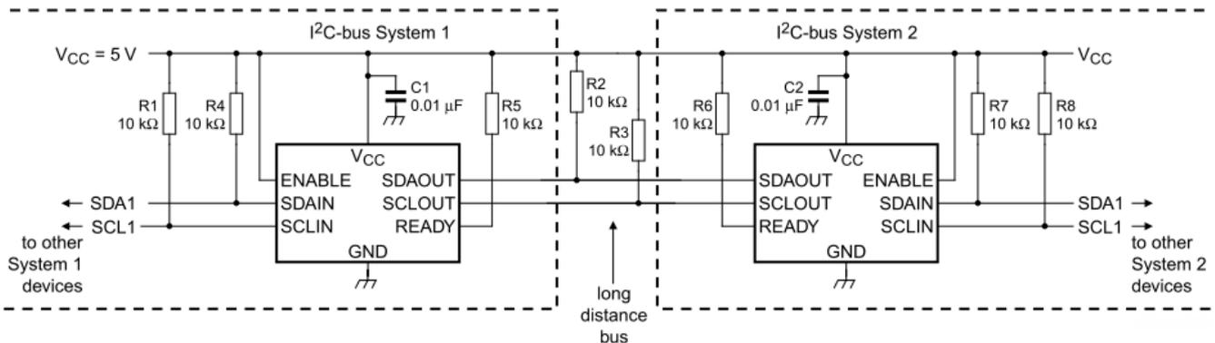
Figure 12. Repeater / Bus Extender Application Using PI6ULS5V9511B
