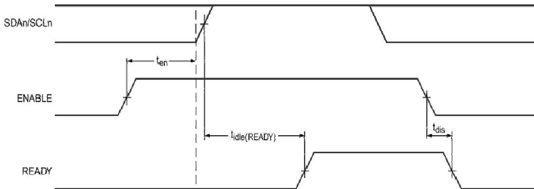
Figure 3. Timing for t<sub>en</sub>, t<sub>idle(READY)</sub> and t<sub>dis</sub>
