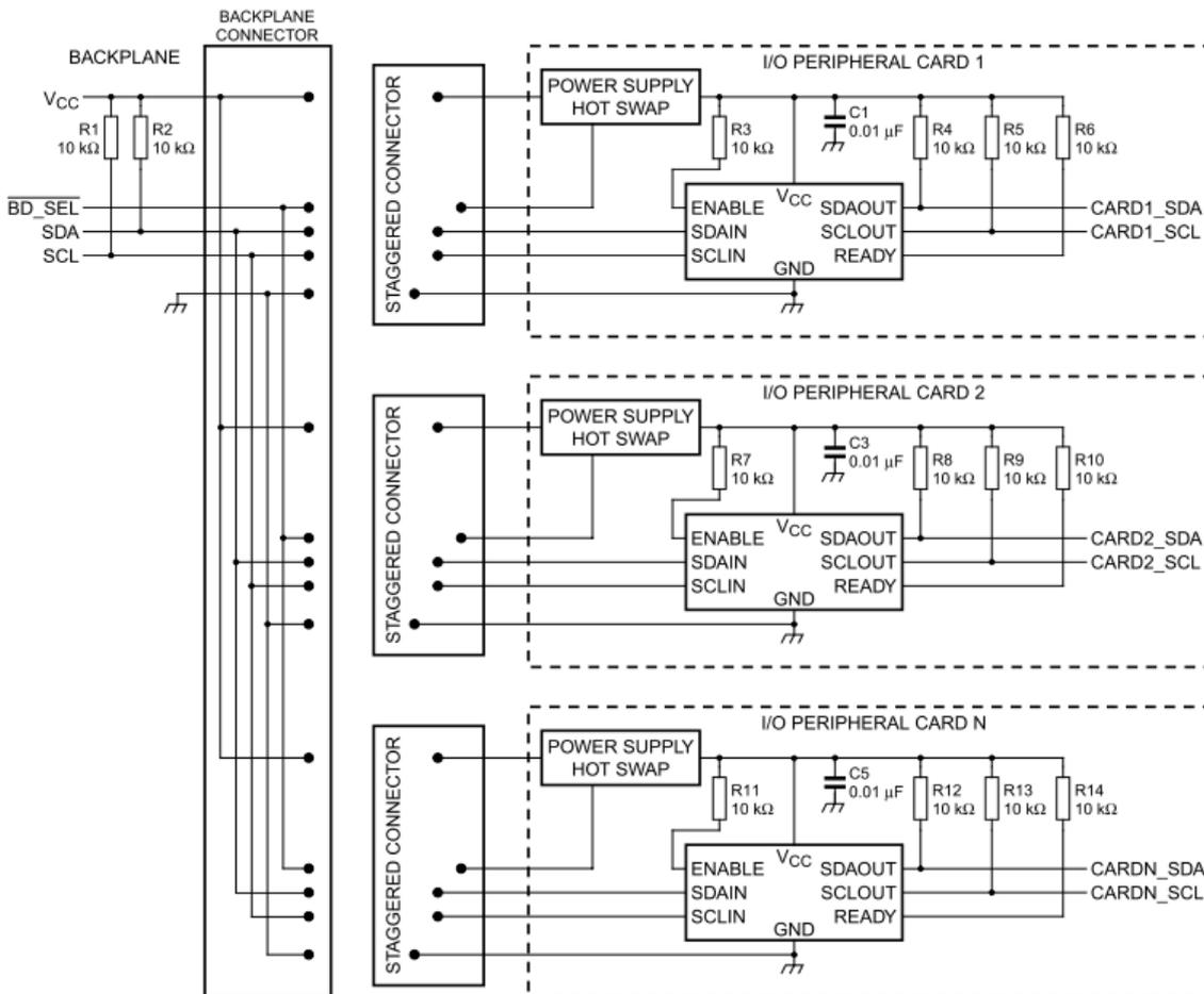
Note: The PI6ULS5V9511B can be used in any combination depending on the number of rise-time accelerators that are required by the system. Normally only one PI6ULS5V9511B is required per bus.
