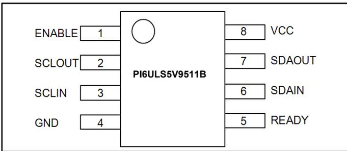
Figure 2. Top View of MSOP-8 and SOIC-8
