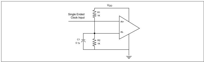
Figure 1. Single-Ended Input to Differential Input Device
