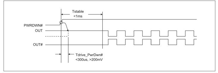
Figure 2. Power down de-assert sequence
