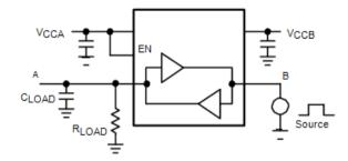
Figure 2. Driving A Test Circuit
