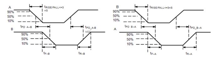
Figure 4. Definition of Timing Specification Parameters
