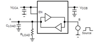
Figure 2. Driving A Test Circuit
