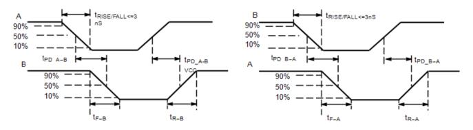
Figure 4. Definition of Timing Specification Parameters
