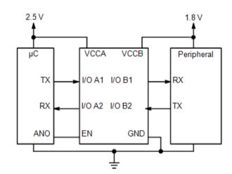
Figure 9 Application Example for A > B
