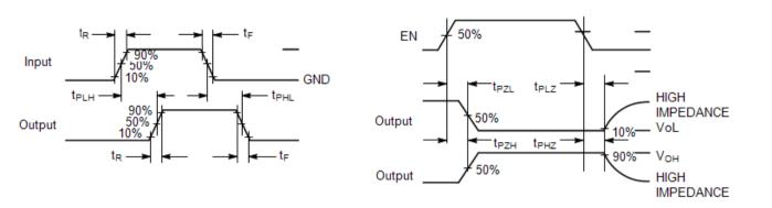
Figure 6. Timing Definitions for Propagation Delays and Enable/Disable Measurement
