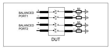
Differential Near End Xtalk Test Circuit
