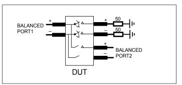
**Differential Off Isolation Test Circuit**
