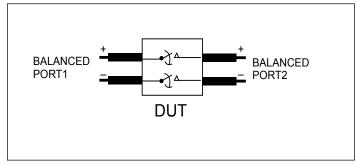
Differential Insertion Loss and Return Test Circuit
