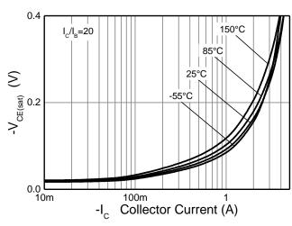
Figure 9. V<sub>CE(sat)</sub> v I<sub>C</sub>
