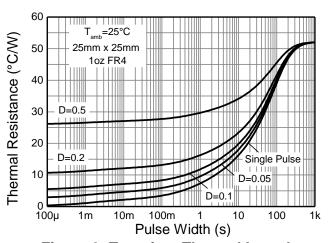
Figure 3. Transient Thermal Impedance
