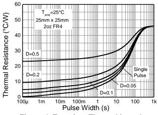
Figure 4. Transient Thermal Impedance
