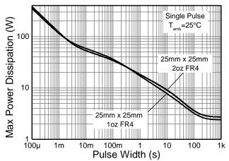
Figure 5. Pulse Power Dissipation
