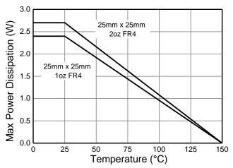
Figure 2. Derating Curve
