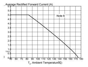
Figure 4. Average Rectified Forward Current vs Ambient Temperature
