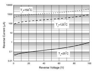
Figure 2. Typical Reverse Current Per Diode
