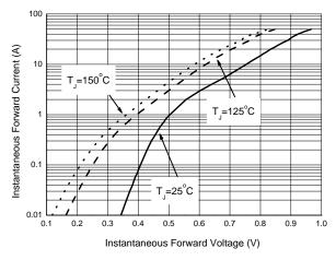
Figure 1. Typical Forward Voltage Per Diode
