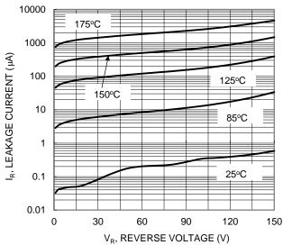
Figure 2. Typical Reverse Characteristics
