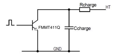
The effect of parasitic inductance in the circuit must be considered. Excessive inductance will reduce the current pulse height and slew current pulse edges. Loop area enclosed by the power circuit and track lengths should be minimized.
