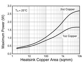
Max Power Dissipation vs. Copper Area
