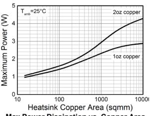
Max Power Dissipation vs. Copper Area
