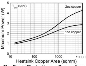
Max Power Dissipation vs. Copper Area
