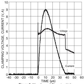
Figure 6. Waveform of Clamping Voltage, Current vs. Time (8/20µs, V<sub>CC</sub> to V<sub>SS</sub>)
