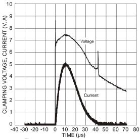
Figure 5. Waveform of Clamping Voltage, Current vs. Time (8/20µs, I/O to V<sub>SS</sub>)
