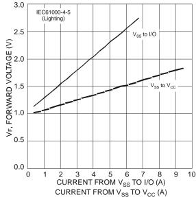
Figure 4. Forward Voltage Characteristics
