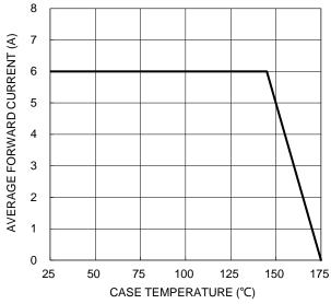
Figure 1. Forward Current Derating Curve
