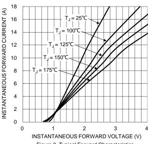
Figure 3. Typical Forward Characteristics
