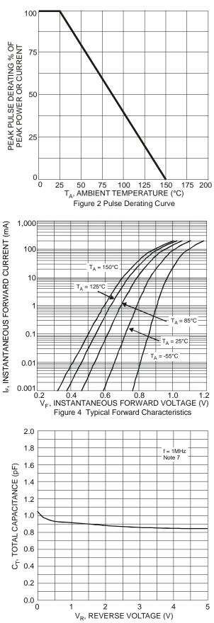
Figure 6 Typical Total Capacitance vs. Reverse Voltage
