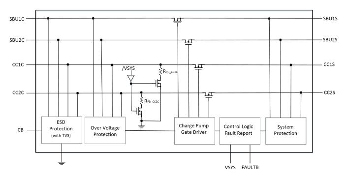
Figure 2. Internal Functional Blocks
