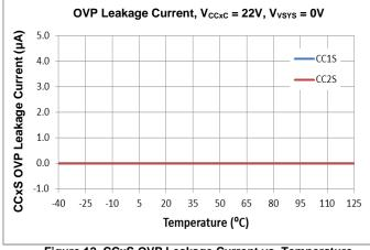
Figure 12. CCxS OVP Leakage Current vs. Temperature
