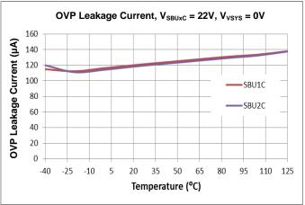
Figure 8. SBUxC 22V OVP Leakage Current vs. Temperature
