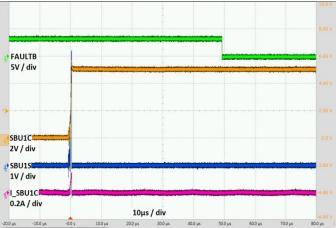
Figure 14. SBU1C Short to 5V V<sub>BUS</sub>
