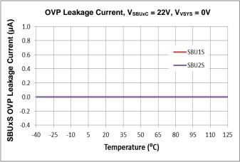
Figure 11. SBUxS OVP Leakage Current vs. Temperature
