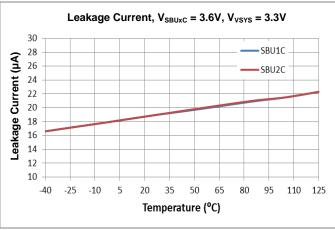
Figure 5. SBUxC Leakage Current vs. Temperature
