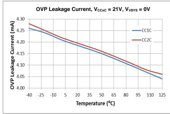
Figure 9. CCxC OVP Leakage Current vs. Temperature
