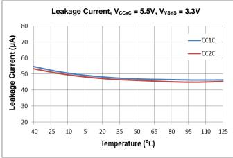
Figure 6. CCxC Leakage Current vs. Temperature
