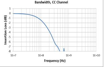
Figure 19. SBU Channel Bandwidth
