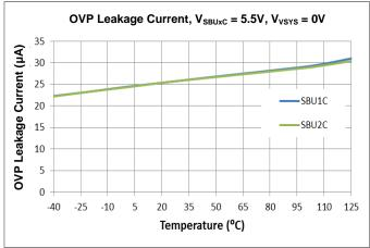
Figure 7. SBUxC 5.5V OVP Leakage Current vs. Temperature
