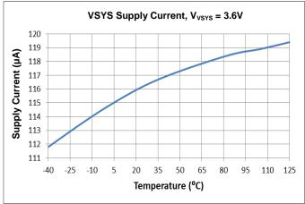
Figure 13. VSYS Supply Current vs Temperature
