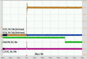
Figure 15. SBU1C Short to 20V V<sub>BUS</sub>
