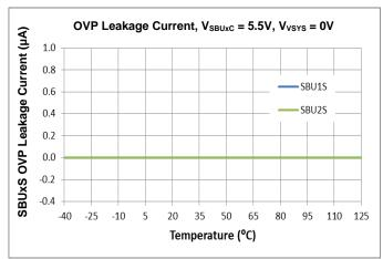
Figure 10. SBUxS OVP Leakage Current vs. Temperature
