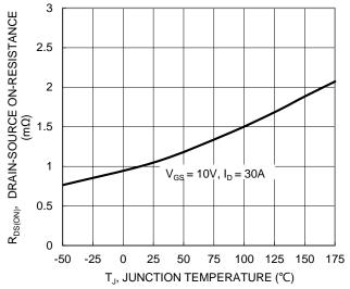
Figure 7. On-Resistance Variation with Temperature
