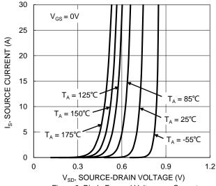
Figure 9. Diode Forward Voltage vs. Current
