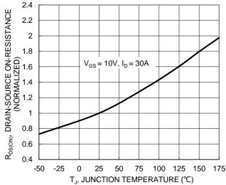
Figure 6. On-Resistance Variation with Temperature
