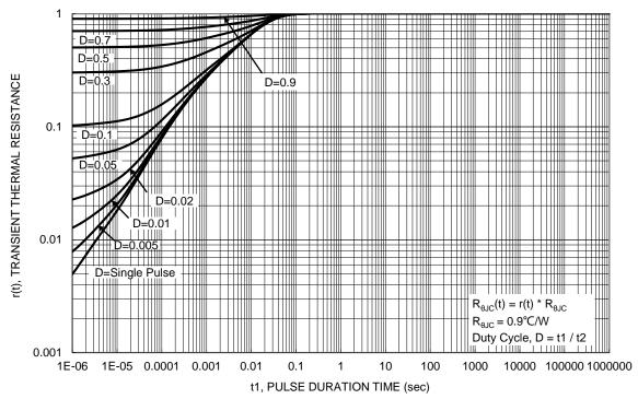
Figure 13. Transient Thermal Resistance
