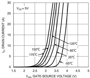
Figure 2. Typical Transfer Characteristic
