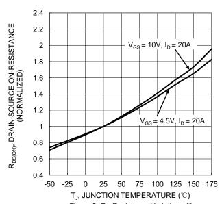
Figure 6. On-Resistance Variation with Temperature
