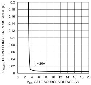
Figure 4. Typical Transfer Characteristic
