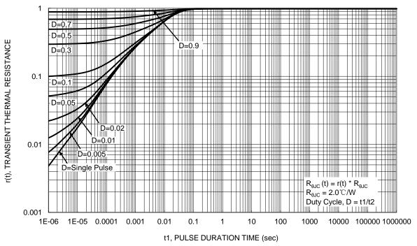
Figure 13. Transient Thermal Resistance
