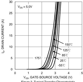
Figure 2. Typical Transfer Characteristic
