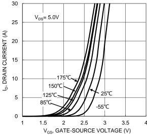
Figure 2. Typical Transfer Characteristic
