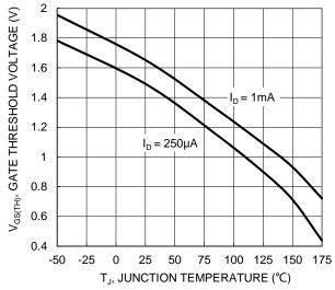
Figure 8. Gate Threshold Variation vs. JunctionTemperature
