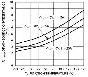
Figure 7. On-Resistance Variation with Temperature
