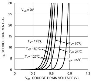
Figure 9. Diode Forward Voltage vs. Current
