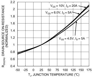
Figure 6. On-Resistance Variation with Temperature
