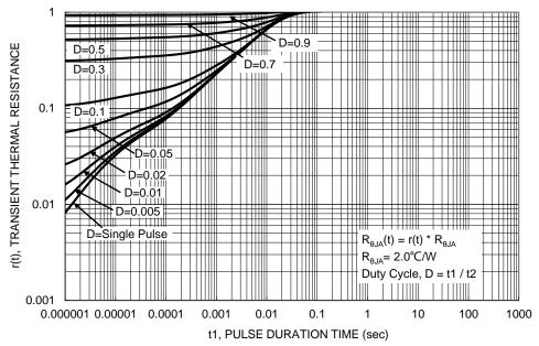
Figure 13. Transient Thermal Resistance
