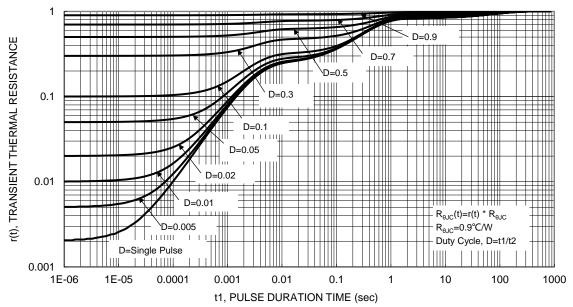
Figure 13. Transient Thermal Resistance
