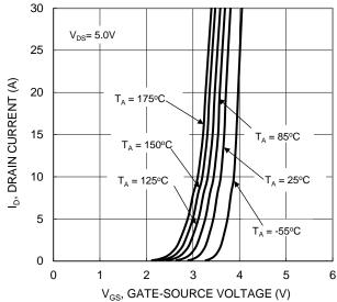
Figure 2 Typical Transfer Characteristic
