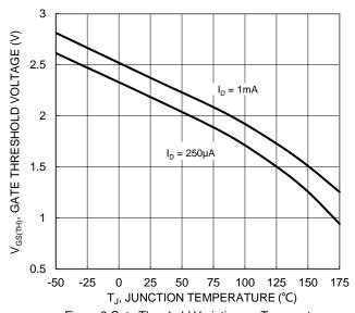
Figure 8 Gate Threshold Variation vs. Temperature
