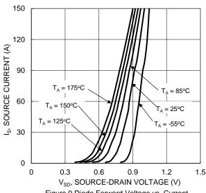
Figure 9 Diode Forward Voltage vs. Current
