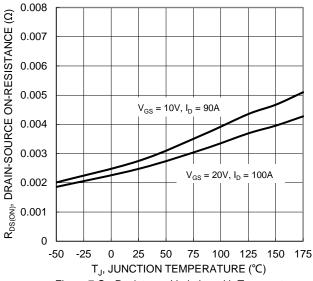
Figure 7 On-Resistance Variation with Temperature
