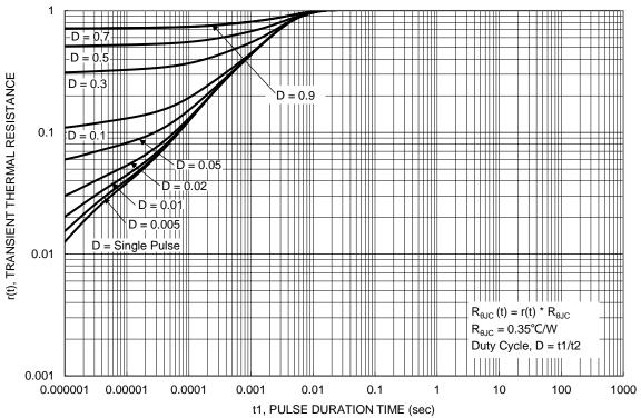
Figure 13. Transient Thermal Resistance
