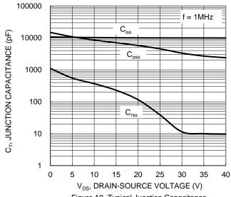
Figure 10. Typical Junction Capacitance
