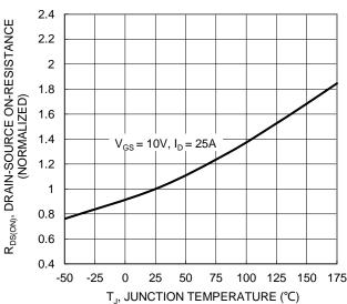
Figure 6. On-Resistance Variation with Junction Temperature
