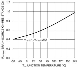
Figure 7. On-Resistance Variation with Junction Temperature
