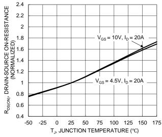
Figure 6. On-Resistance Variation with Temperature
