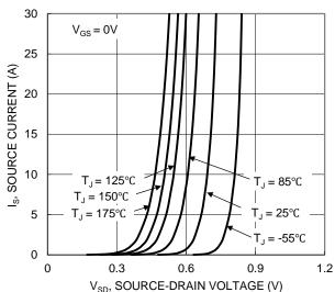
Figure 9. Diode Forward Voltage vs. Current
