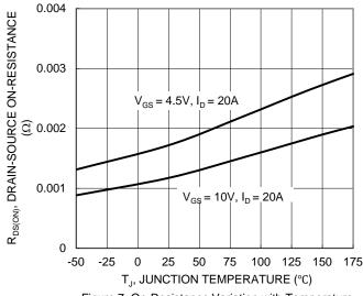
Figure 7. On-Resistance Variation with Temperature
