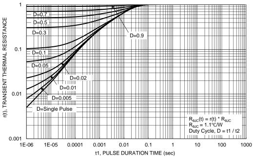
Figure 13. Transient Thermal Resistance
