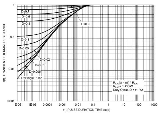
Figure 13. Transient Thermal Resistance
