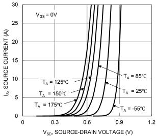
Figure 9. Diode Forward Voltage vs. Current
