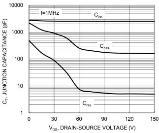
Figure 10. Typical Junction Capacitance
