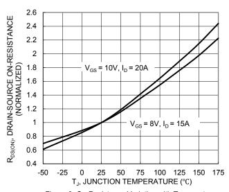
Figure 6. On-Resistance Variation with Temperature
