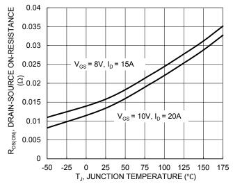
Figure 7. On-Resistance Variation with Temperature
