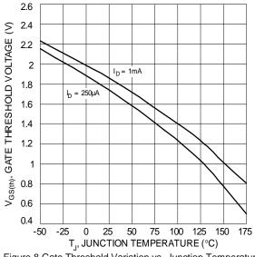
Figure 8 Gate Threshold Variation vs. Junction Temperature
