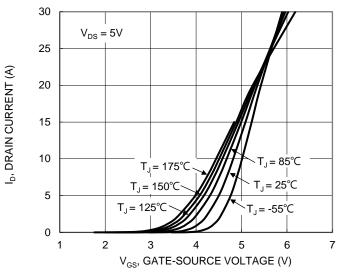
Figure 2. Typical Transfer Characteristic
