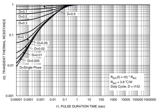
Figure 13. Transient Thermal Resistance
