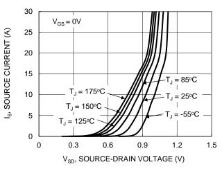
Figure 9. Diode Forward Voltage vs. Current
