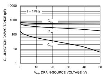
Figure 10. Typical Junction Capacitance
