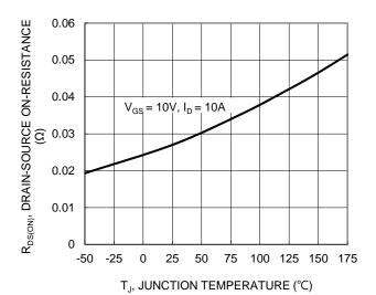
Figure 7. On-Resistance Variation with Junction Temperature
