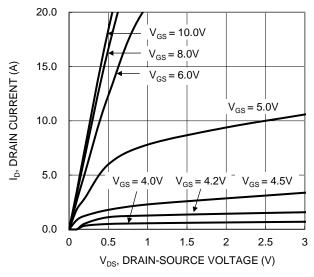
Figure 1. Typical Output Characteristic
