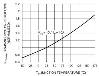
Figure 6. On-Resistance Variation with Junction Temperature
