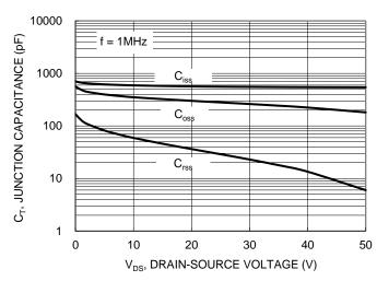
Figure 10. Typical Junction Capacitance
