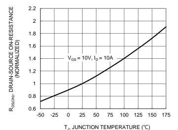
Figure 6. On-Resistance Variation with Junction Temperature
