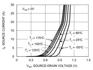
Figure 9. Diode Forward Voltage vs. Current
