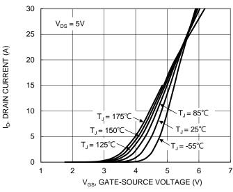
Figure 2. Typical Transfer Characteristic
