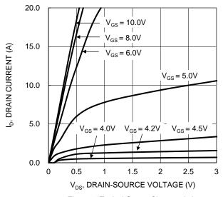
Figure 1. Typical Output Characteristic
