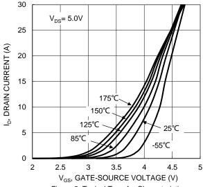
Figure 2. Typical Transfer Characteristic
