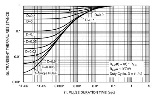
Figure 13. Transient Thermal Resistance
