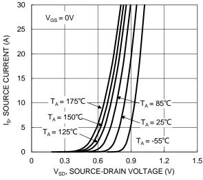
Figure 9. Diode Forward Voltage vs. Current
