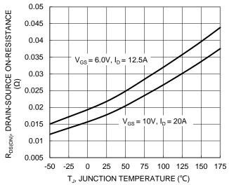
Figure 7. On-Resistance Variation with Temperature
