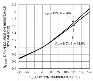
Figure 6. On-Resistance Variation with Temperature
