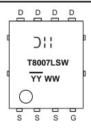
) | | = Manufacturer's Marking T8007LSW = Product Type Marking Code  $\overline{YY}$ WW = Date Code Marking  $\overline{YY}$  = Year (ex: 22 = 2022) WW = Week (01 to 53)
